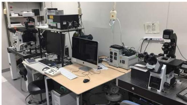
**Widefield deconvolution microscopes with high-precision motorized XYZ stages and home-built adaptation to create limited-area high-intensity laser light for DNA damage or FRAP studies.**
