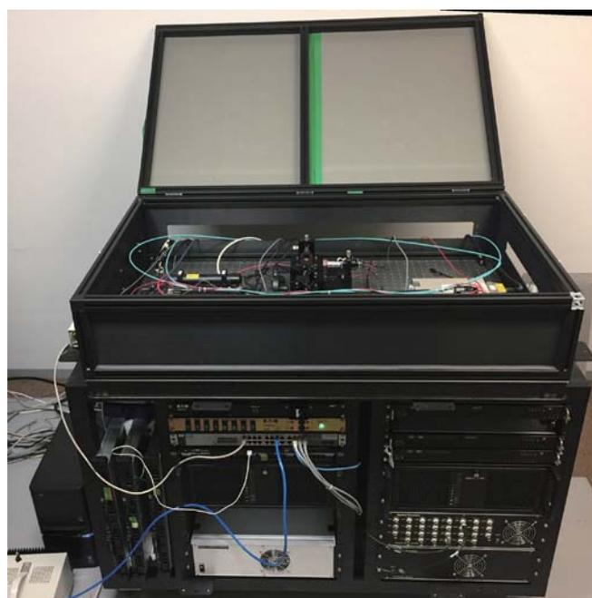
Laser light source, control, and processing unit for the OMX 3D-SIM superresolution microscope.
